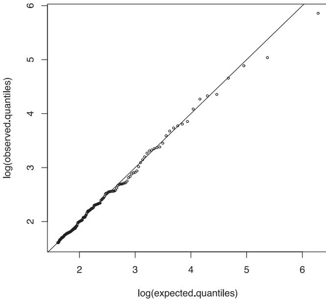
FIGURE 5: QQ plot of fire data on log-log scale, assuming a Pareto(500, 1.209) model.
